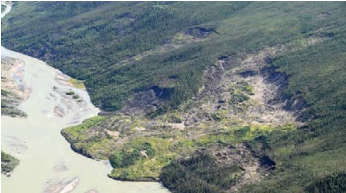
Figure 18. Recent slope instability associated with permafrost thaw, including active layer detachment slides and retrogressive thaw slumps. In the foreground, large amounts of material have pushed into the river to form a debris tongue. Foothills of the Mackenzie Mountains south of Norman Wells, north-western Canada. Credit: Government of Northwest Territories, Canada.
